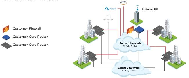
CPE routers managed by the carrier terminate MPLS/VPLS or Layer 2 Ethernet circuits at each customer site into a customer's routed environment and connect back to the Provider Edge (PE) router in the carrier's network. The PE allocates bandwidth and provides features such as QoS as the packets are transported across the carrier network using VRF or VLAN to other circuits connecting the carrier network to the targeted cloud providers and/or data centers.
