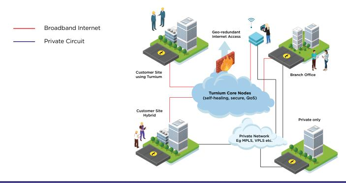
An SD-WAN network with centralized and secure Internet access can be deployed to connect multiple existing sites, including offices and data centers.
